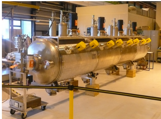
RF module with 8 RF cavities in series.
