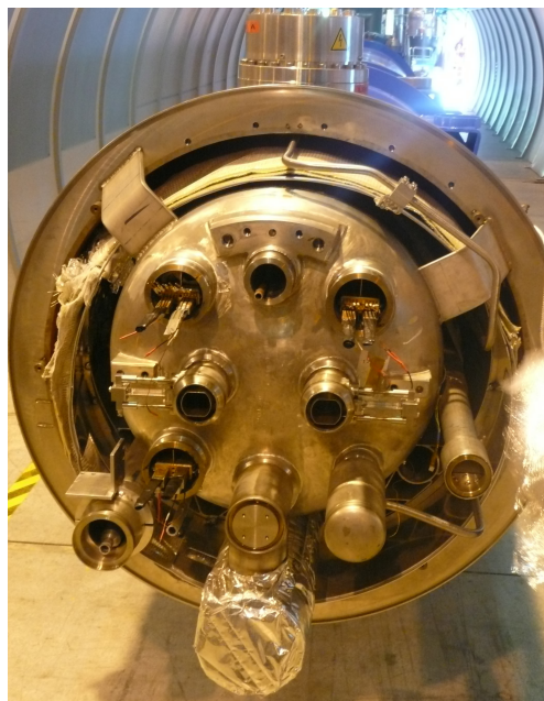
End view of magnet, with beam tubes (centre) and helium pipes.
