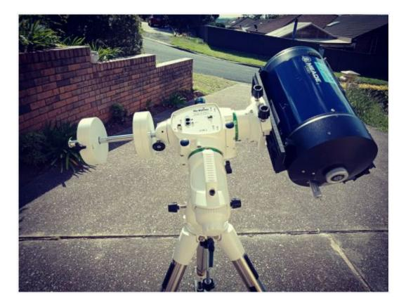
The Esprit, (840mm focal length), gives me images of  $1.5^{\circ} \times 1.0^{\circ}$  using the ZWO ASI071 but the LX-90 (2000 mm) gives me images of about 38' x 25' using the same camera. It gave me larger images of planets, planetary nebulae and galaxies.
