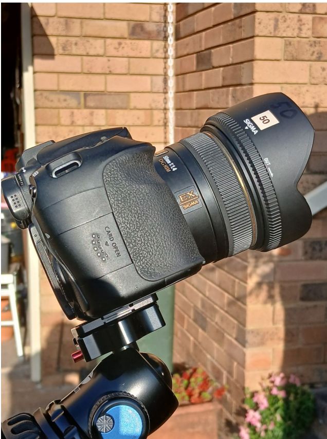
DSLR camera and ball head attached to the main axis of the Star Adventurer body.
