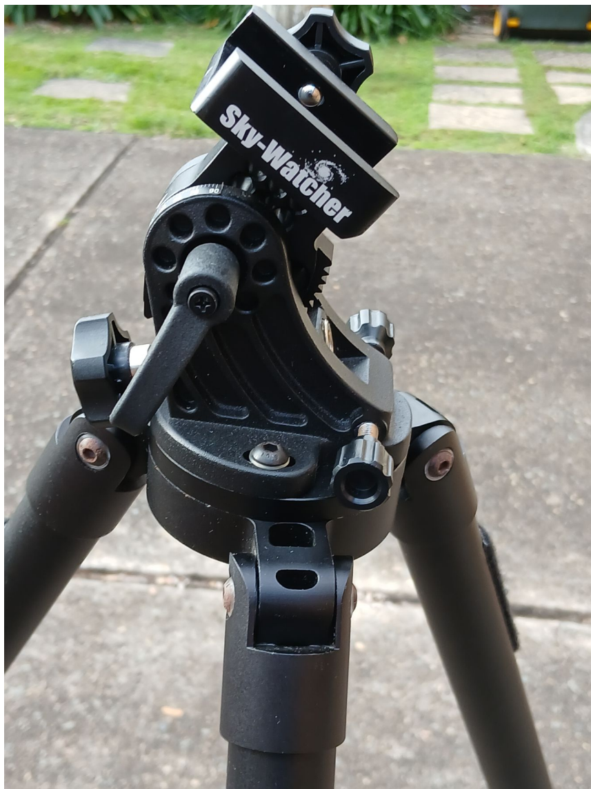
The Wedge fitted to the tripod, showing the altitude knob (left) and the two azimuth knobs (right).
