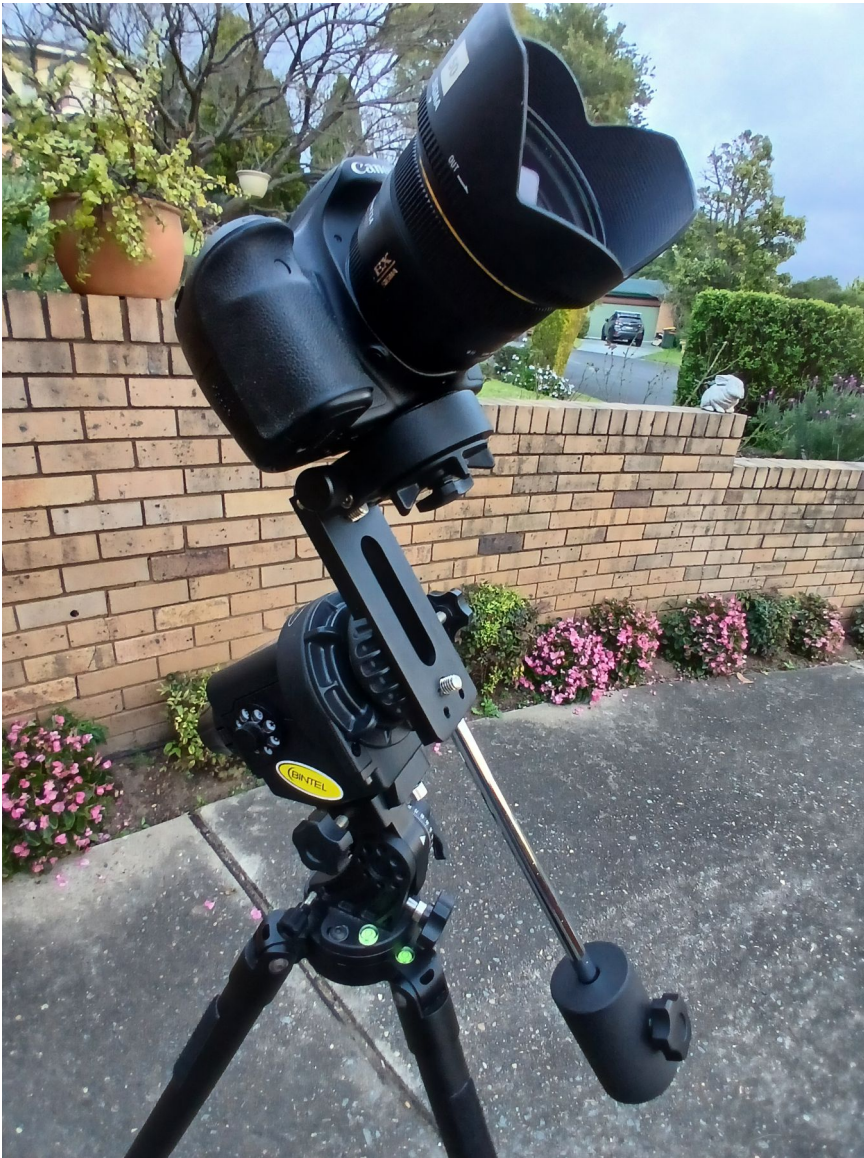
The Star Adventurer with the fine tuning mounting assembly installed. Ready to go!
