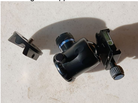
The dovetail connector (left) and a Sirui ball head with arca Swiss mount female attachment.
