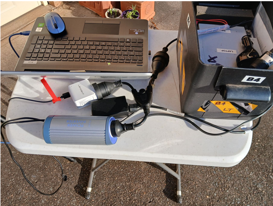
Figure 2: 2024-09-18 Star Adventurer Laptop controller, powered by 12 volt battery. Rear view, showing 12V DC to 24V AC inverter (blue ends) and 240V distribution to standard laptop inverter (black) and 5V USB power (white) to dew heater.
