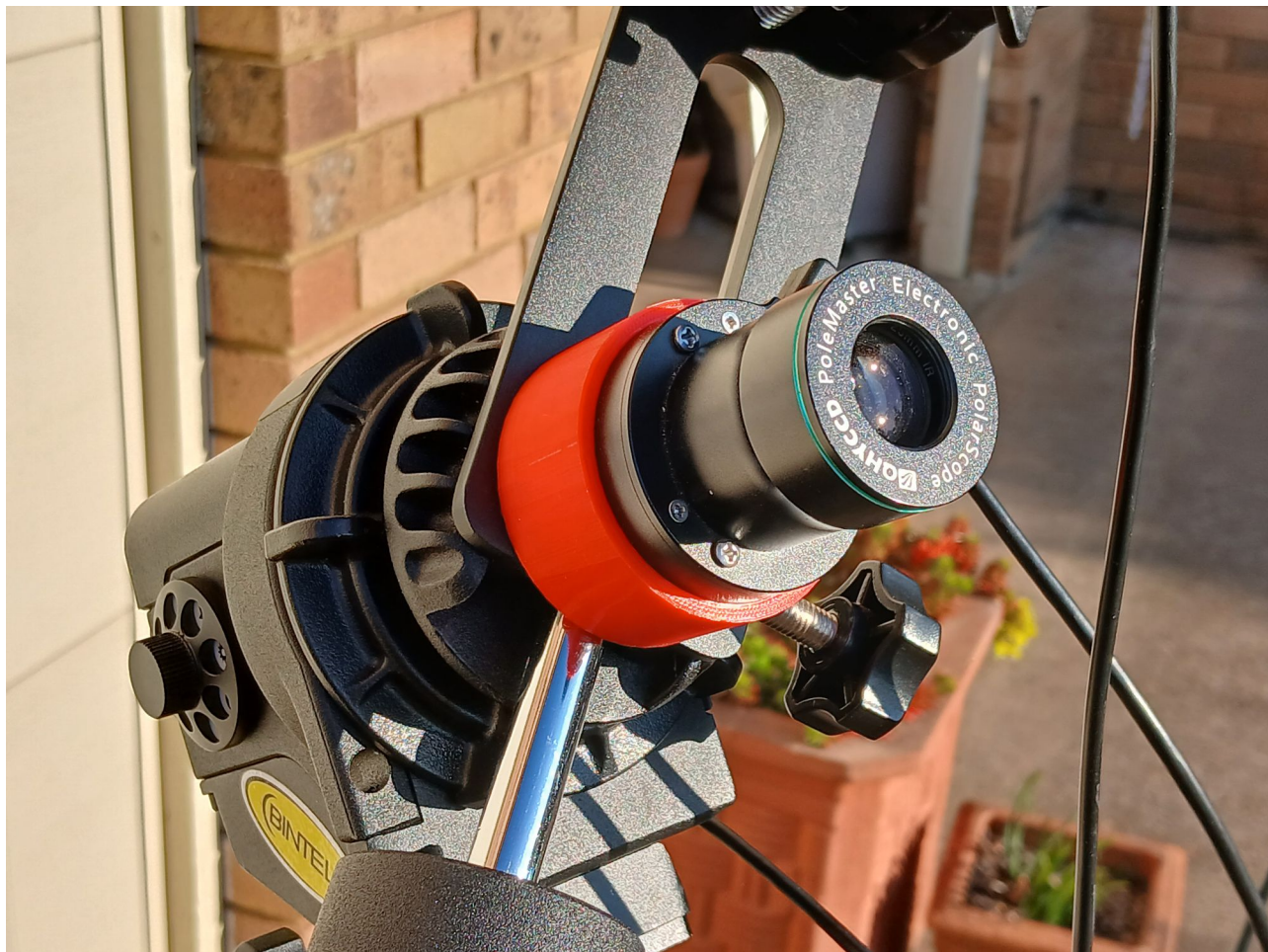
Figure 4: The PoleMaster camera provides a wide angle view of the Celestial Polar region, to provide accurate polar alignment.
