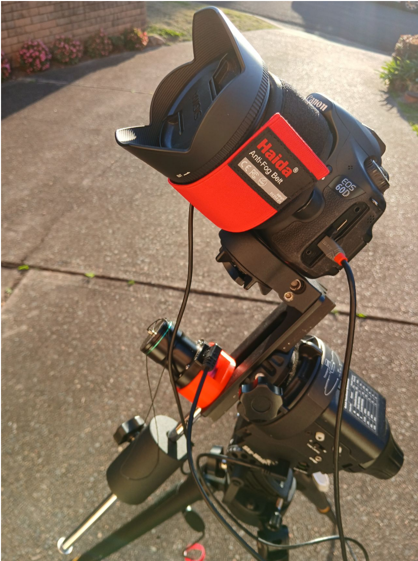
Figure 3: DSLR with Dew Heater mounted on the Star Adventurer .Note also the PoleMaster camera mounted parallel on the Fine Tuning Mounting Assembly
