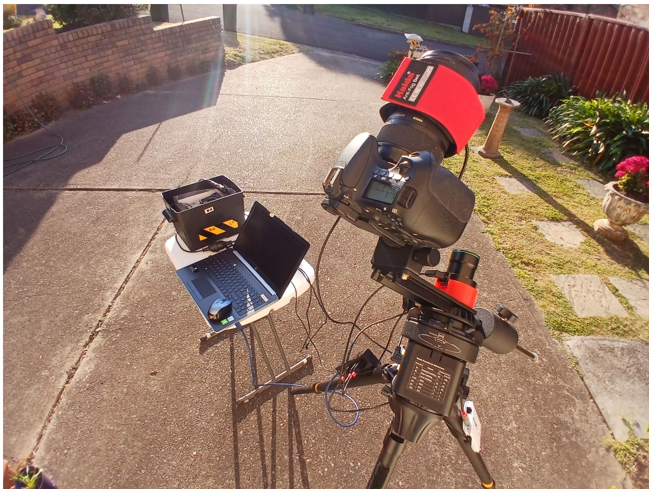
Figure 9: An elevated view of the wired up Star Adventurer , with laptop and power supply alongside.
