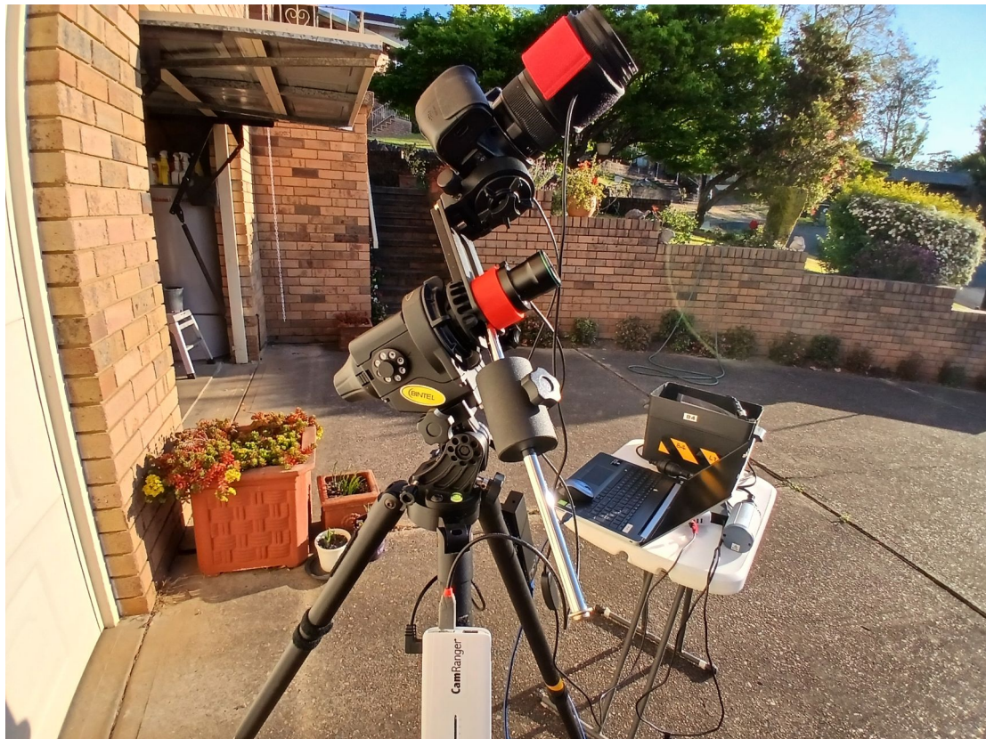
Figure 8: The Star Adventurer wired up, with lap top and power supply on adjacent table.
