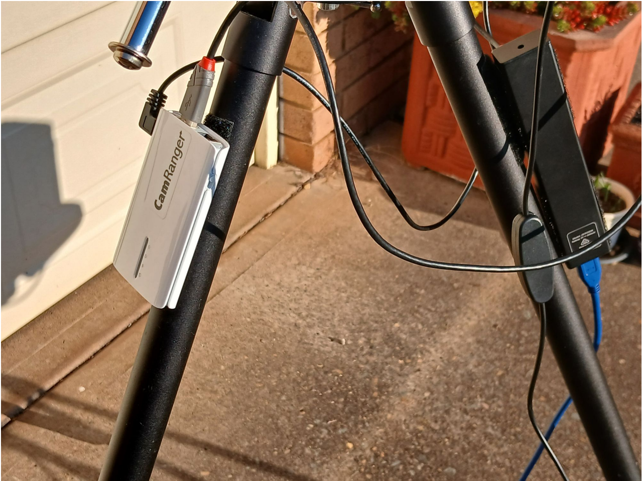
Figure 5: The Cam Ranger wired up for 5 volt power(black connection), image control and acquisition (Red/grey connection).
